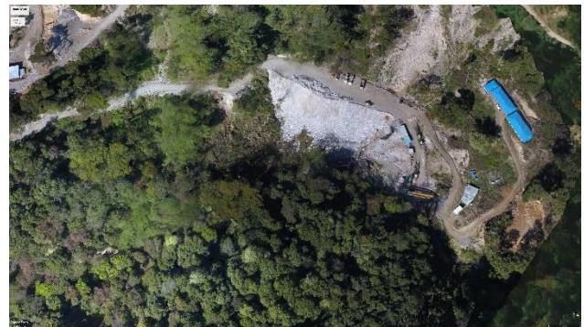
Figure 20.2: Forest area cleared in patches during development of muckyard at Adit-II
